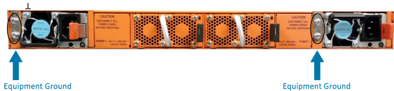
Figure 7 Ground Screws (GigaVUE TA Series Shown)
